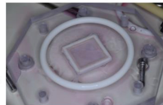
Decellularized tissue aligned in tissue holder part
