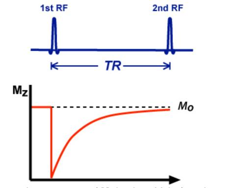
When TR >> T1 there is complete recovery of  $M_z$  back to  $M_o$  before the 2nd RF-pulse.
