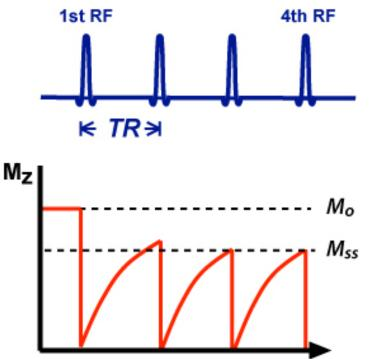
When  $TR \leq T1$ , partial saturation occurs with development of steady-state magnetization  $M_{ss} < M_o$ .
