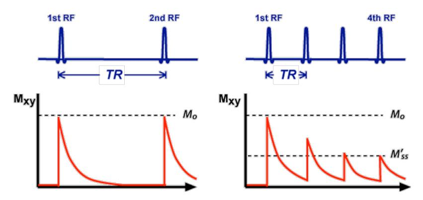
TR  $\leq$  T2 and Mxy does not fully decay to zero before next RF-pulse is applied. After a few  $_{\odot}$  pulses a new nonzero steady-state transverse magnetization (M'ss) is reached.
