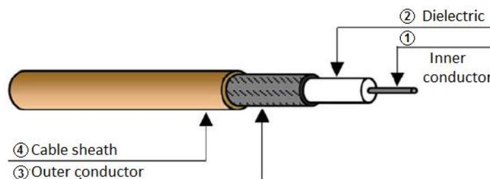
Fig. 1 Coaxial cable RG -178.
