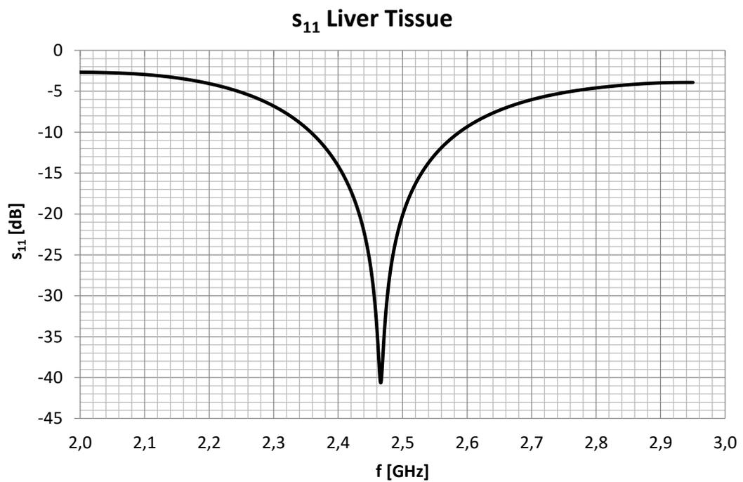
Fig. 9.: Resulted  $|S_{11}|$  curve.
